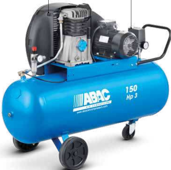
A39 150 CM3 3 hp, 100 litres, lubricated
