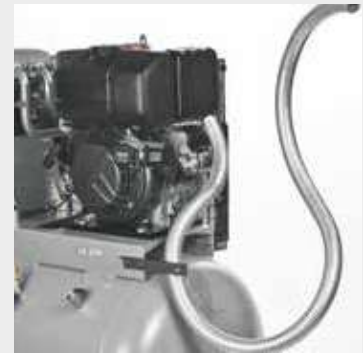
Exhaust extension Kit for indoor use or in closed motor vehicles*
